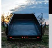
A sturdy 2" square tubing top rail, 24" tall 10-gauge sides and a single-piece, 10-gauge steel floor create a durable dump box.
