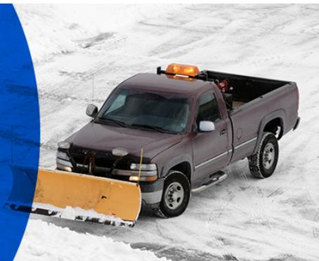
Plows come in many shapes and sizes and are designed to scoop and push snow to the side to clear a road. The DOT might use a 12-foot-wide reversible plow, for example, to clear a 10-foot-wide path. The operator maneuvers the plow from inside the cab using levers or a controller.
